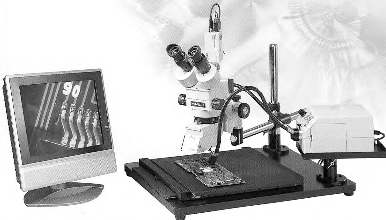
SMD INSPECTION SYSTEM : EMZ-8TR Zoom stereo microscope, F Focus block, MA797 oblique viewing attachment, MA503 Super widefield 15X eyepieces, UL universal stand, MA574 sliding stage, FL151 dual arm 150W fiber optic illumination system, MA151/5N video "C" mount, CK3900 video camera and video monitor.
